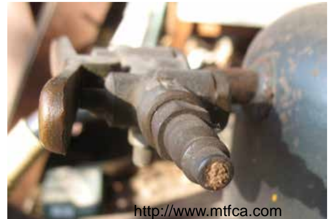
Mud wasp nest in valve of Model T Ford
